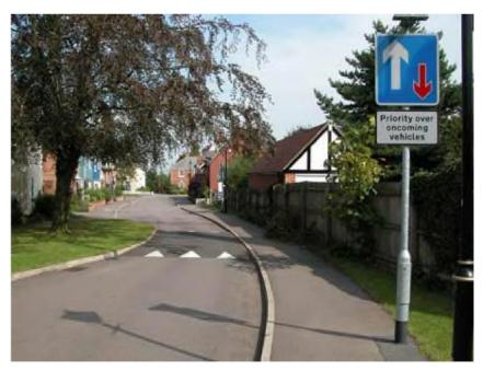
Figure GL3 Example of a shuttle-working speed control feature
