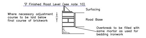
10. All ironwork to be set so that the frames and covers finish flush with adjacent finished road level. On gullies, the frames and covers should either be flush or up to 6mm below the finished road surface to assist in drainage of the carriageway.
